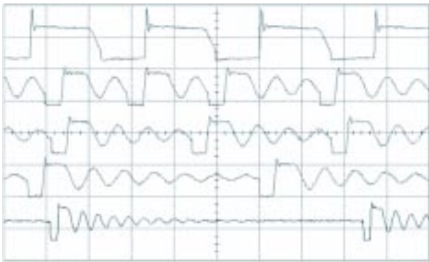
Figure 8. Typical operating waveforms for different output powers down to no-load operation (bottom curve)
