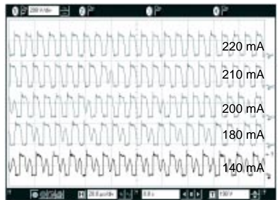
Figure 7. Multiple pulses start to occur further to the transition into VCO control
